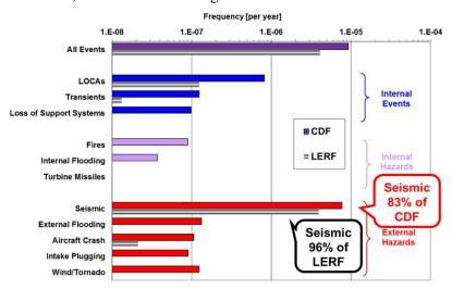
Figure 3 Core damage frequency (CDF) und Large early releases frequency (LERF) at Beznau NPP (Status 2015)(RICHNER 2015)
