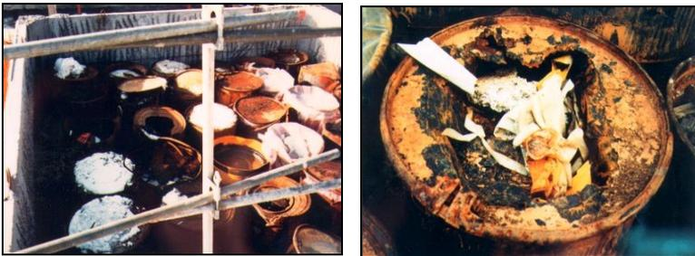
*Damaged and leaking waste barrels inside CSM*
