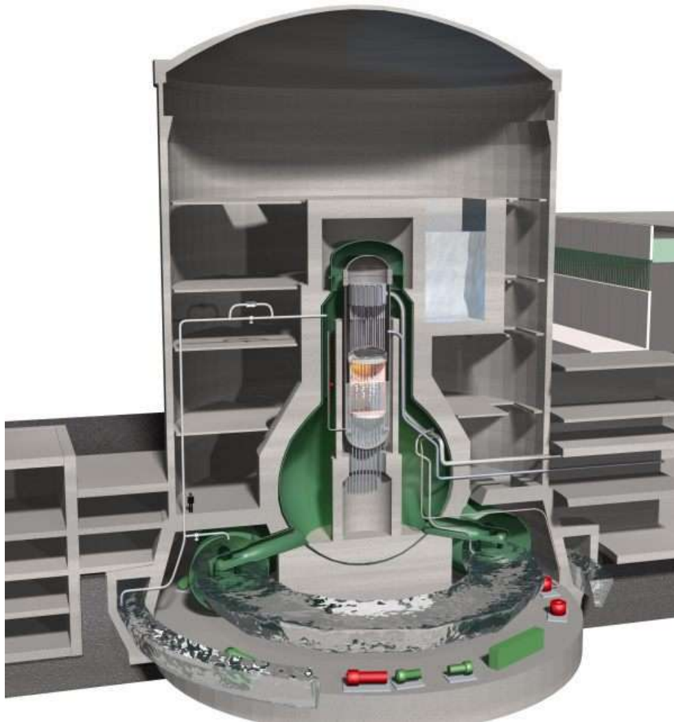
Figure 3: KKM Mark 1 Containment [Source: KUEHNI 2011]
