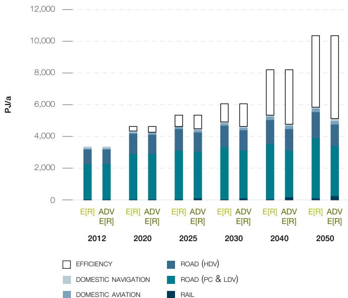
FIGURE 6.5.3 | AFRICA: DEVELOPMENT OF THE FINAL ENERGY DEMAND FOR TRANSPORT BY SECTOR IN THE ENERGY [R]EVOLUTION SCENARIOS
