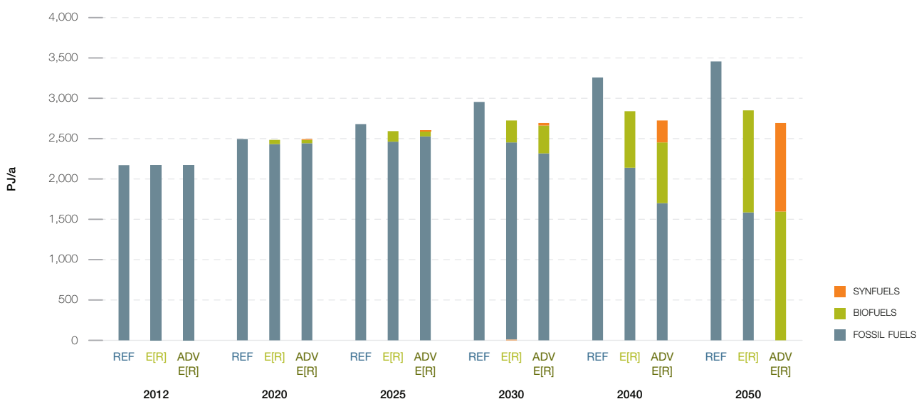
FIGURE 12.11 | DEVELOPMENT OF FINAL ENERGY USE FOR MARINE TRANSPORT BY TECHNOLOGIES IN THE REFERENCE AND BOTH ENERGY [R]EVOLUTION SCENARIOS
